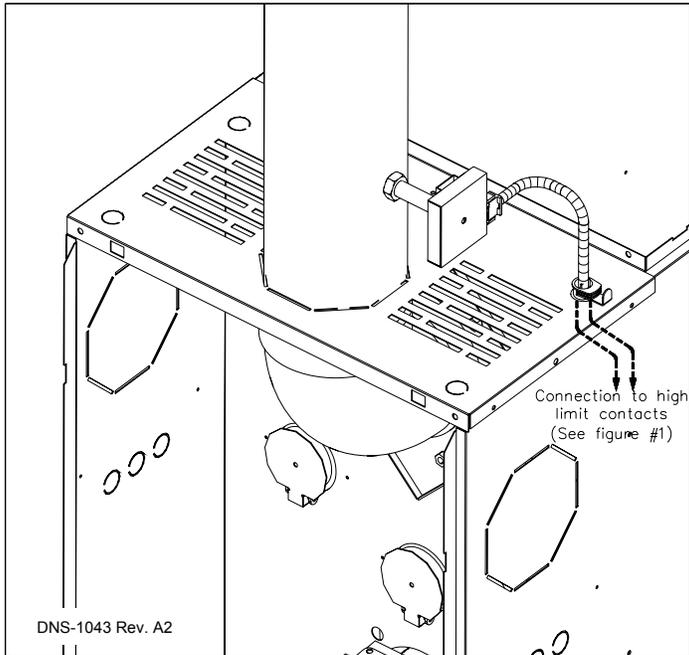
**Blocked Vent Shut-Off device wiring
