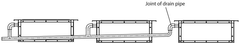
The specification of the joint of the drain pipe should be suitable to the running capacity of the unit.
