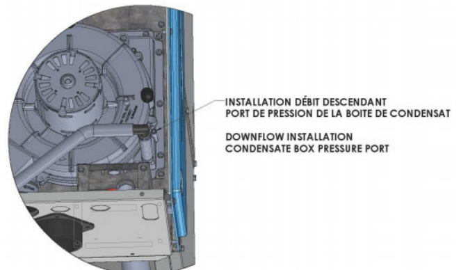
Figure 8: Downflow condensate box pressure port
