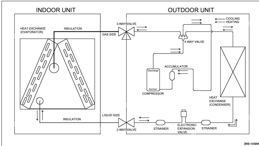
\* Properly insulate **ALL** refrigerant tubing from outdoor units to the interior cooling coil to prevent water dripping.
