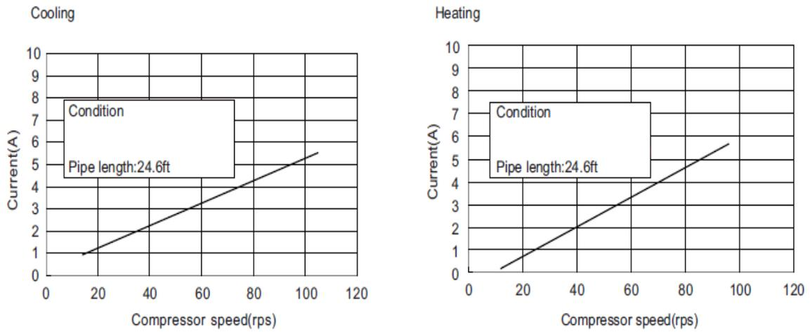
Figure 2: 12K Operation characteristics curves
