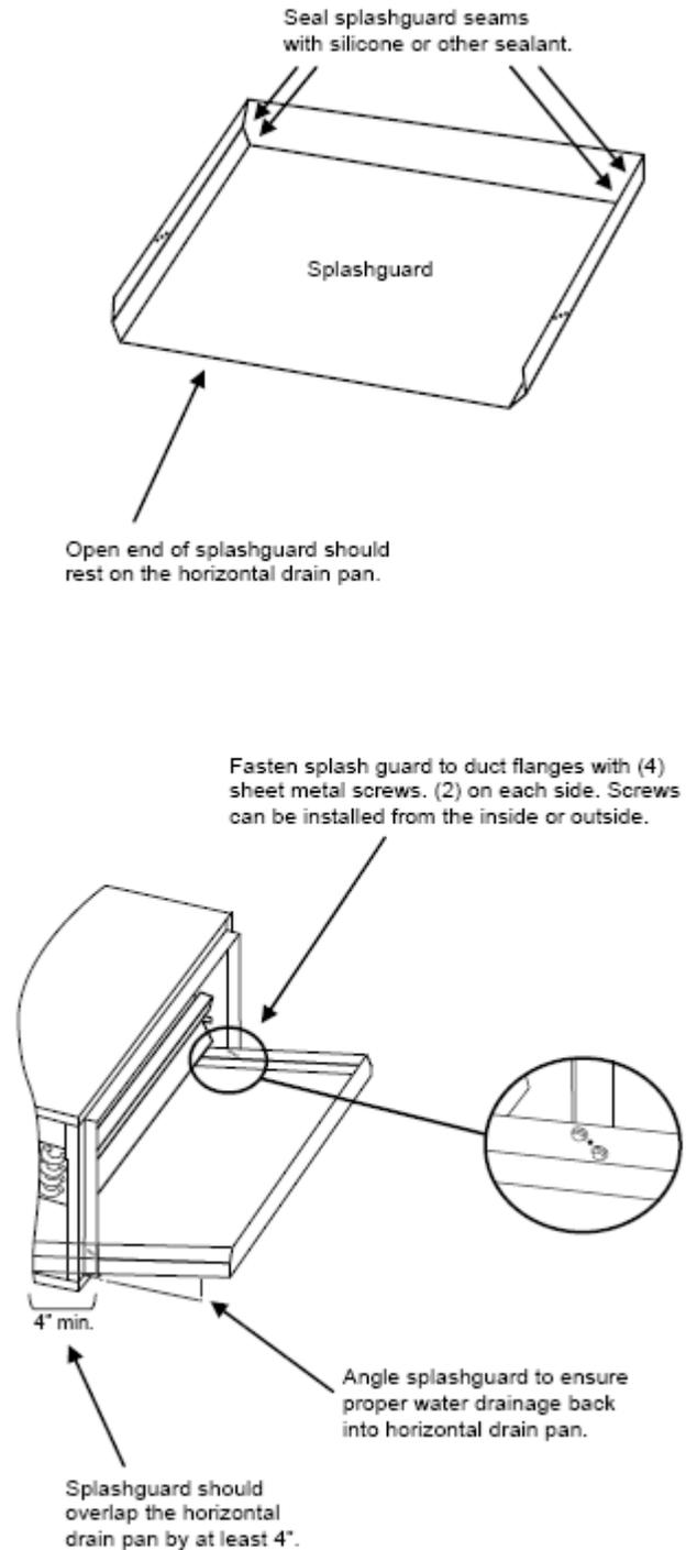
Figure 22: Splashguard with front slope
