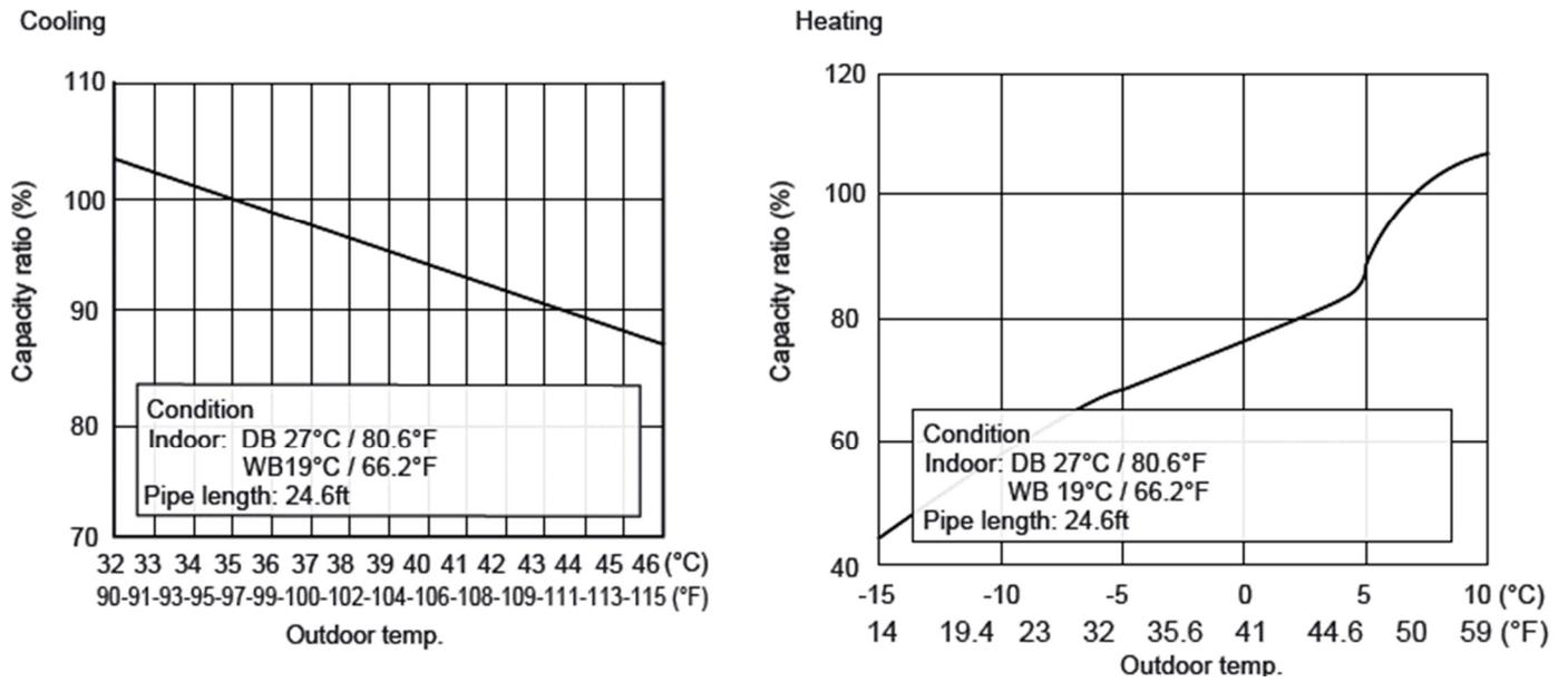
Figure 5: 18/24K Capacity ratio vs outdoor temperature
