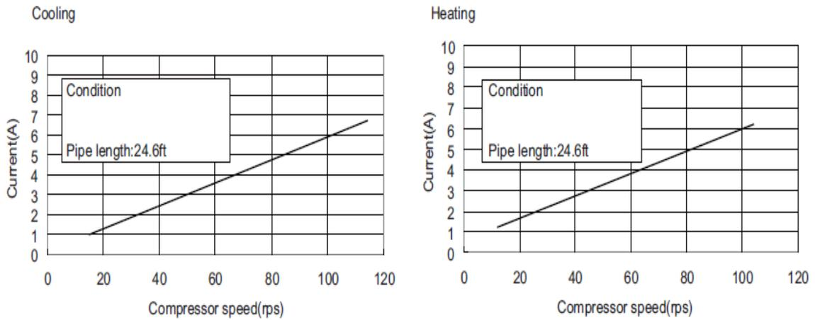
Figure 3: 18/24K Operation characteristics curves
