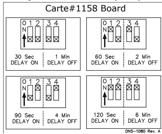
start/stop delays of the blower must also be adjusted by positioning the DIP switches on the electronic board as shown in the following figures. For upflow installation, the recommended blower ON delay is 60 seconds and blower OFF delay 2 minutes.
