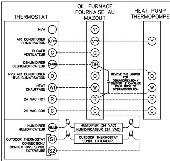
**Note:** On units with 2-stage cooling or heat pump, terminal Y1 must be used. When Y1 on the electronic control receives a 24 VAC signal, the airflow is reduced by 20%. Do not use terminal Y1 with a single stage cooling or heat pump.
