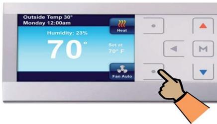
**Fan Auto** This is the most commonly used setting. The fan will turn on only when the heating or cooling system is running.
