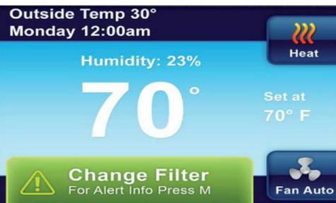
Your thermostat can automatically provide reminders when the air filter, humidifier pad, or UV lamp needs to be replaced. Each of these reminders are turned on or off and the reminder time period set from the appropriate item in the Thermostat Settings Menu (section 3.11).
