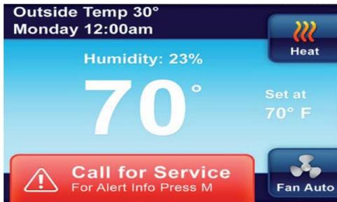
If the thermostat senses trouble with a component of your system (the heat pump, air handler, furnace or air conditioner), or a maintenance reminder appears, an alert will be displayed on the Home screen. Details of any alert can be found on the **Alert Info Detail** menu in the main menu. Your installing dealer contact information may also be displayed on this screen.
