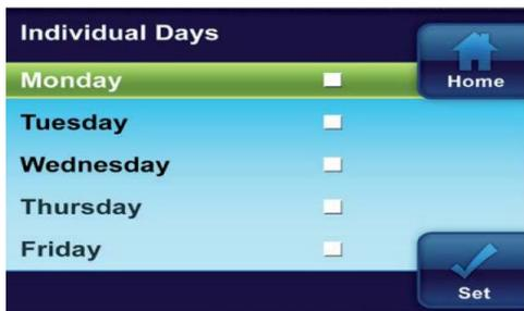
Using **Individual Days** allows you to change the program settings of a single day or days. Highlight a day and press **M** to mark the box. Mark additional days you wish to have programmed the same. Press **Set** to begin entering the program for the selected day or days.
