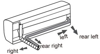
2. When selecting leading out the pipe from left or right, please cut off the corresponding hole on the bottom case.
