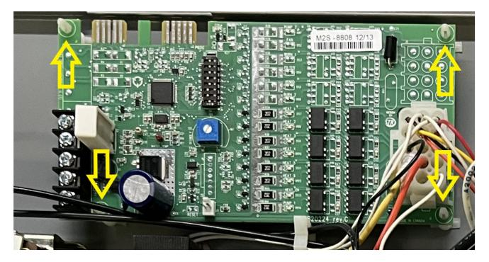
5. Take out the new control board and connect the water temperature sensor to it.
