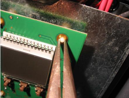
3. Disconnect the defective control board
