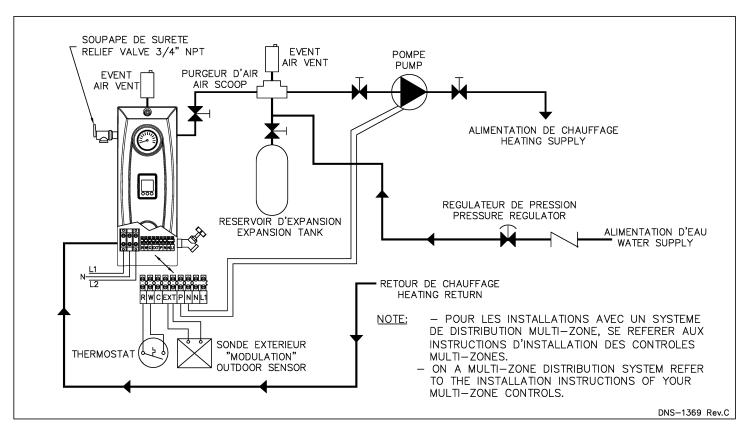
Figure 7: Typical Diagram of a Single Zone Installation
