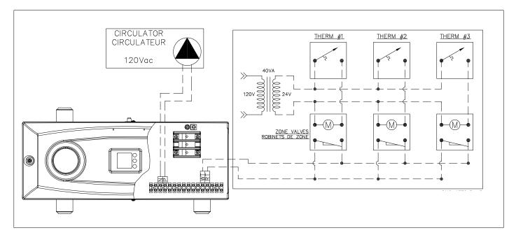
Figure 10: Dual-energy Installation
