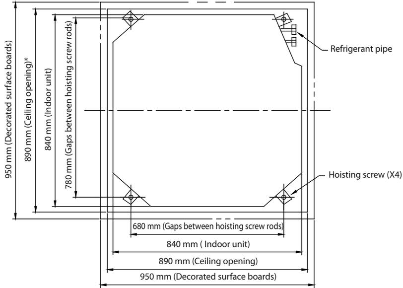
\*This dimension could be as large as 910 mm as long as the overlapping section of the ceiling and the decorated surface boards is no less than 20 mm.
