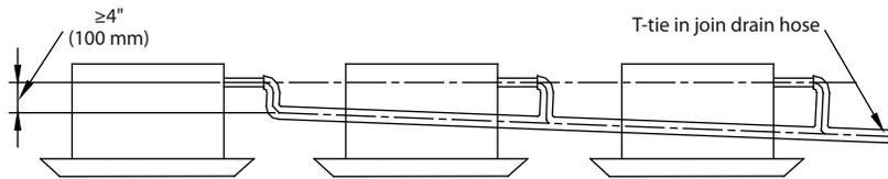
The specification of the drain pipe joint should be suitable to the running capacity of the unit.
